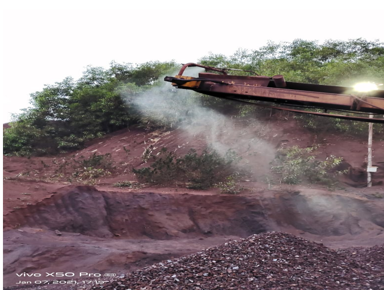
Dry Fog System in Mineral Handling Plants
